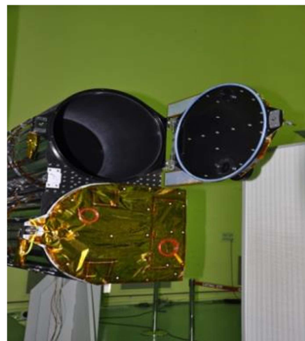
Figure 4b: UV Telescope cover Deployment in Lab
