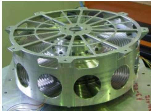
Figure 7: SSM Steering Mechanism
