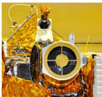
Figure 5: SXT Cover Deployed condition
