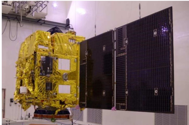
Figure 2: Deployed Solar Array during ground tests.
